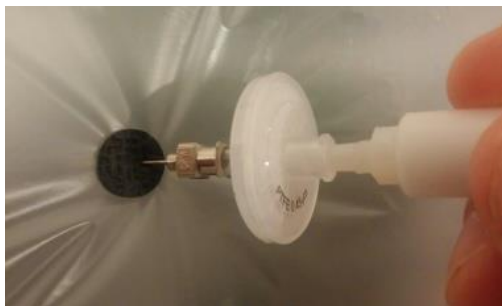
Sampling from a package using the PTFE filter, needle, and foam septa.
